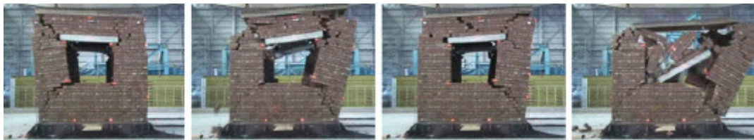
Process of specimen collapse in the shaking table test
