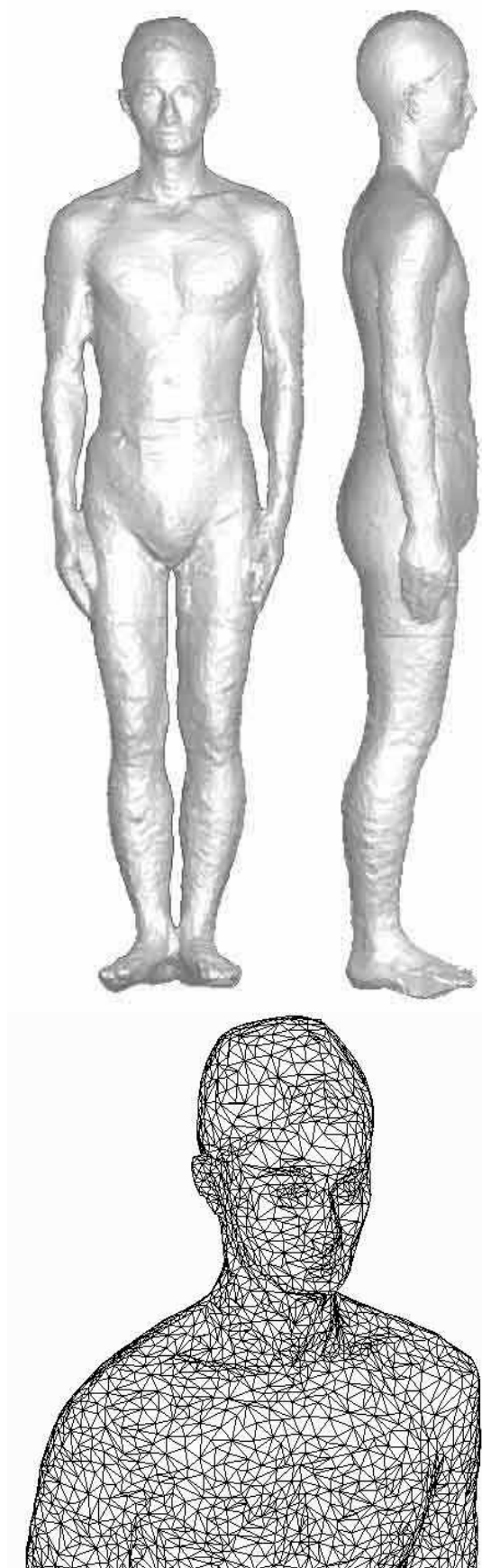
Fig. 1 Three-dimensional human body surface simulation model.
