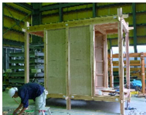
Photo. 2 Higher timber frame specimen.
